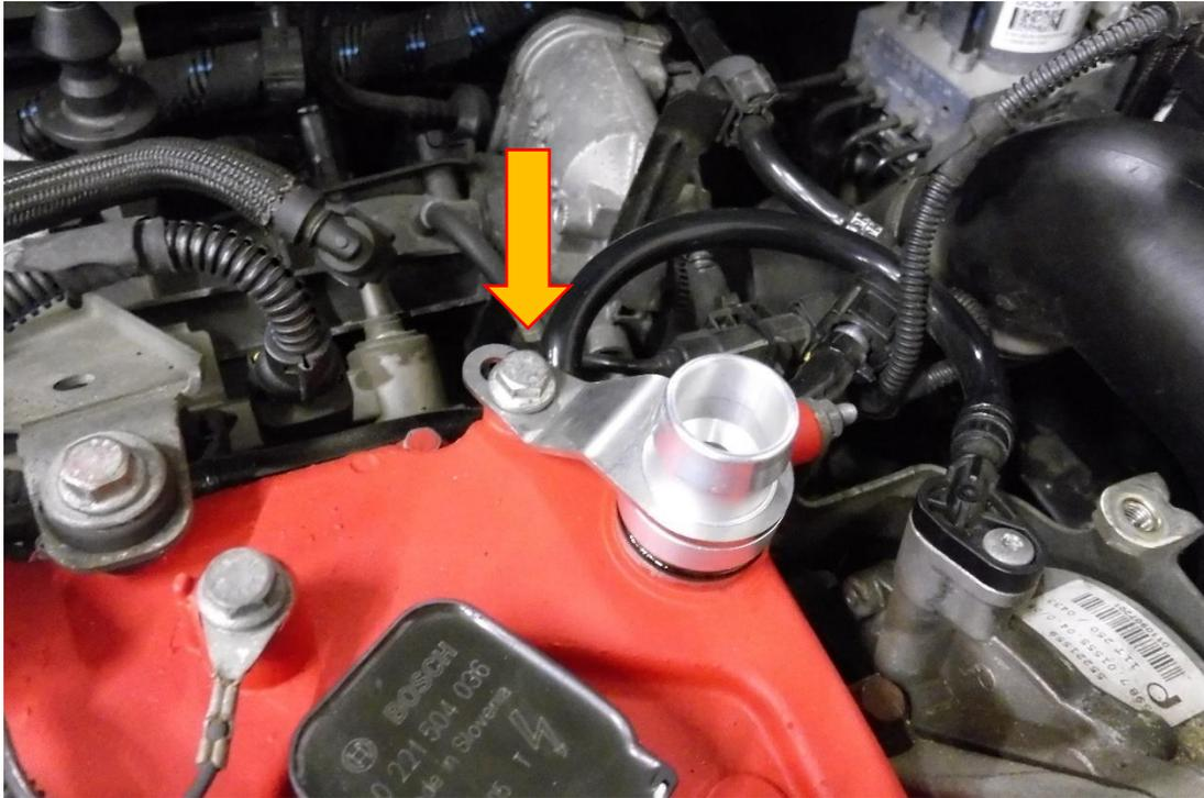
11. Using a 7mm socket and ratchet secure the silicone blank to the redundant spout on the inlet manifold.
