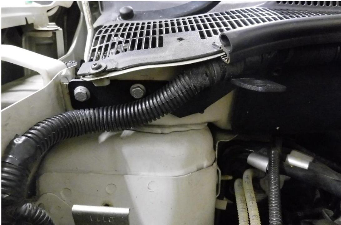
8. Re fit the brake fluid reservoir, just slide it back into place.
