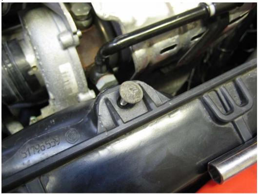
2. Remove the four hoses on the pipe between the airfilter and the turbo, as indicated below (the engine cover does not need to be removed), then remove the pipe from the turbo and pull it out of the airbox to remove it from the car.
