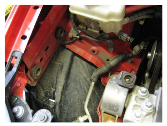
4. Using a pair of needle nosed pliers, remove the cotter pin in the turbo housing.
