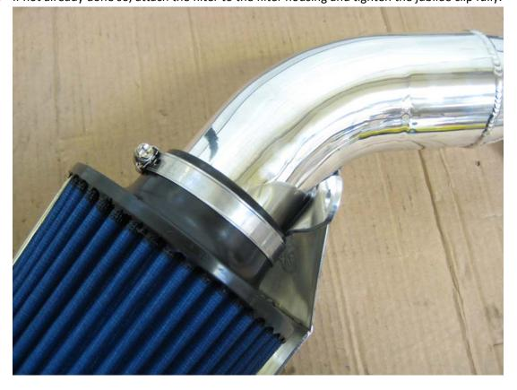
8. Place the filter assembly into the silicon joiner already on the turbo.....
