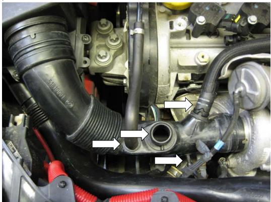
3. Pull up on the side of the airbox nearest the engine as shown below to remove it from the grommet, then pull it towards the engine to remove it from the two grommets in the inner wing.
