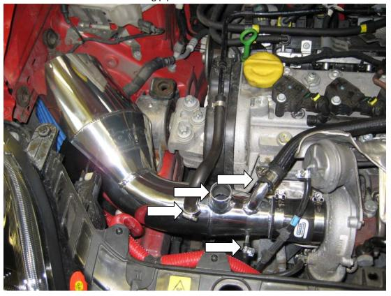
10. When everything is lined up OK, first tighten the 10mm nuts on each side of the rubber damper, then both jubilee clips holding the filter assembly to the turbo, then each of the four hoses in turn. Installation is complete!
