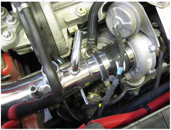
$\dots$  and locate the bracket under the filter onto the other end of the rubber damper, fitting an M6 nut to secure it loosely
